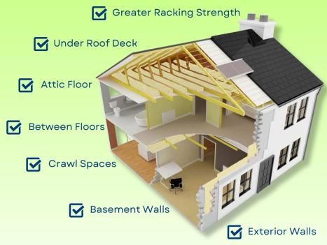
Spray Foam Insulation in Exterior Walls provides a thermal barrier that prevents leaks and keeps indoor temperatures stable. Spray foam insulation in exterior walls also functions as a sound barrier and significantly cuts down on noise intrusion.
